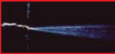
Injector spray pattern before P.i. treatment
