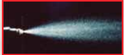
Injector spray pattern after P.i. treatment
