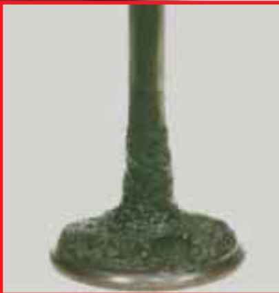
Intake valve before P.i. treatment
